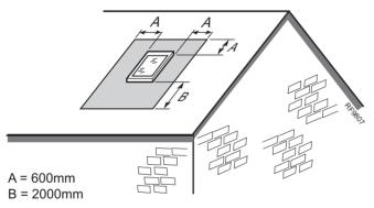
The flue terminal shall not penetrate the shaded area of the roof
