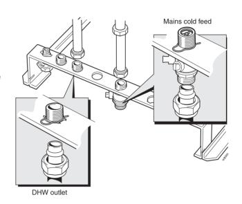
The PRV (pressure reducing valve) provided in the hardware pack MUST be fitted in a convenient point on the mains cold inlet to the appliance. Once fitted, a pressure balanced cold feed to mixer taps and showers may be taken downstream of the PRV but before the istor appliance.
