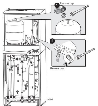
Check the pre-charge pressures on both expansion vessels and top up if necessary.
