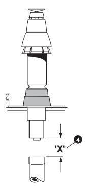
**4.** If the last extension duct requires cutting, measure 'X', the distance (outer ducts), between the duct and the terminal and add 100 mm to this dimension. This gives the length of the last extension duct.
