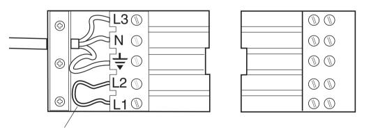
Remove link when connecting external programmer.
