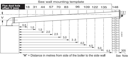
**Note.** If wall thickness is greater than 305mm then dimension "**H**" must be reduced by the same amount and the offset may be adjusted accordingly.
