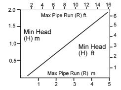
The above graph assumes 8 elbows in the gravity circuit. For each elbow in excess of 8, (R) must be reduced by 300 mm (12 in.) or (H) increased by 100 mm (4 in.)
