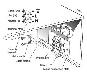
**Note.** If an optional programmer is to be fitted refer to the instructions provided with the kit and Frame 19.
