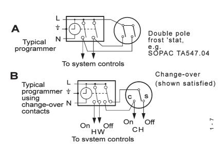
Central heating systems fitted wholly inside the house do not normally require frost protection as the house acts as a 'storage heater' and can normally be left at least 24 hrs. without frost damage. However, if parts of the pipework run outside the house or if the boiler will be left off for more than a day or so, then a frost 'stat should be wired into the system.
