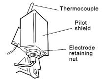
**4.** Unscrew the central pilot fixing screw and lift the pilot burner clear of the thermocouple and pilot injector.
