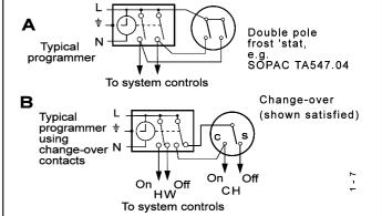
Central heating systems fitted wholly inside the house do not normally require frost protection as the house acts as a 'storage heater' and can normally be left at least 24 hrs. without frost damage. However, if parts of the pipework run outside the house or if the boiler will be left off for more than a day or so, then a frost 'stat should be wired into the system.
