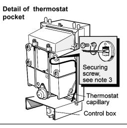
5. Remove the control box fixing screw and pull the box forward and downward to disengage.
