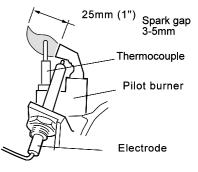
set to maximum and no further adjustment should be necessary. However, if the pilot flame appears small, check the pilot injector. Refer to Frame 39.
