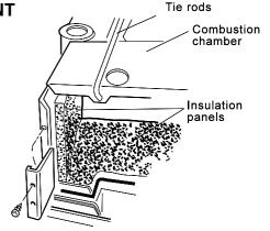
**Detail of boiler combustion chamber**
