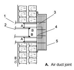
B. Flue duct joint
