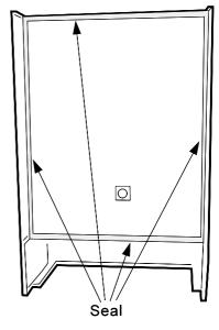
Inner view of boiler casing
