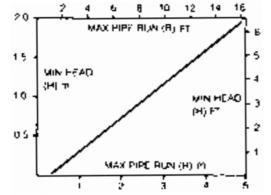
The above graph assumes 8 elbows in the gravity circuit. For each elbow in excess of 8, (R) must be reduced by 300 mm (12 in.) or (H) increased by 100 mm (4 in.)
