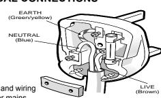
All external controls and wiring MUST be suitable for mains voltage. Wiring should be in 3-core PVC insulating cable
