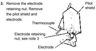
4. Unscrew the central pilot fixing screw and lift the pilot clear of thermocouple and pilot injector.
