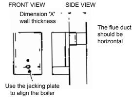
The wall must be of suitable load-bearing capacity
