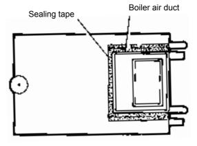
**Note:** Do not remove the controls protection box until the boiler has been lifted onto the wall mounting plate.
