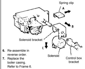
Check the function of the gas control valve
