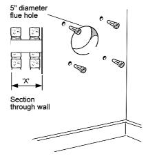
Note. Check all of the hole positions BEFORE drilling
