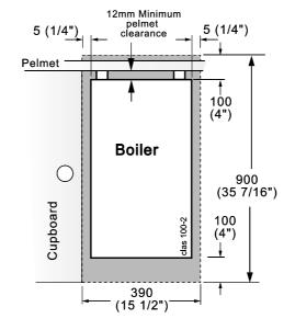
Front clearance: 533mm (21") from the front of the boiler casing.
