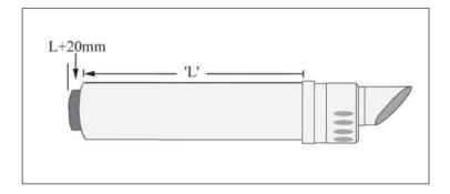
**10.14** The vertical system diagram is shown in *figure 17*. Maximum flue length is 5 m for vertical and 4 m for horizontal. Remember that the diaphragm should be removed for flue length over 1 m.
