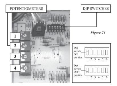
The potentiometers can be reached by removing the cover on the rear of control panel (*Figure 22*). But to reach the dip switches, the control panel must be opened.
