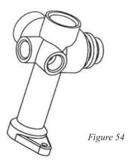
Open isolating valves on flow and return connections, refill, vent and pressurise boiler ensuring all joints are sound.
