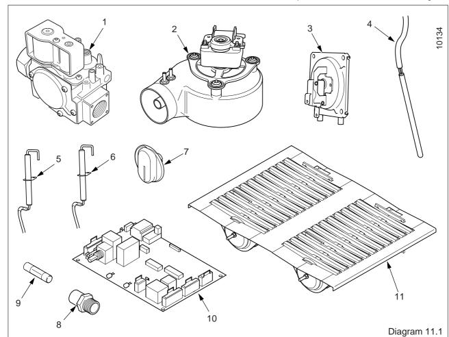
GC Part No. Key No. Part No. Description 2000461898 1 Multifunctional control 2 227132 Fan 2000227137 3 Air pressure switch \*\*\*\*\* 4 2000461793 Electrical thermistor 5 202635 Ignition electrode (R/H Burner) Sensing electrode (L/H Burner) 202635 6 7 2000461714 Boiler temperature control knob 2000461897 Injector CFF100 8 8 205746 Injector CFF115 9 202240 Fuse 10 2000461896 Control board 205657 Double Burner \*\*\*\*\* 11
