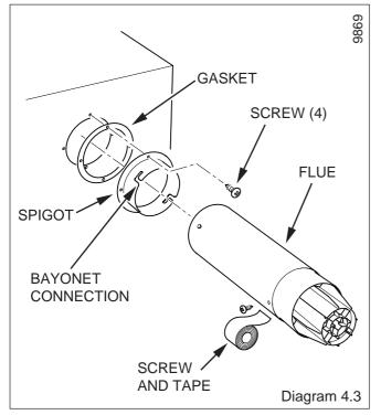
Make sure that the ductings do not slope down towards the boiler.
