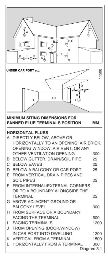
Car ports or similar extensions of a roof only, or a roof and one wall, require special consideration with respect to any openings, doors, vents or windows under the roof. Care is required to protect the roof if it is made of plastic sheeting. If the car port consists of a roof and two or more walls, seek advice from the local gas company before installing the boiler.
