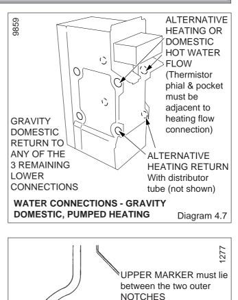
MUST BE IN PUMPED RETURN CONNECTION UPPER MARKER Diagram 4.8 DISTRIBUTOR TUBE 9859 **ALTERNATIVE** FI OW POSITIONS (must be adiacent to THERMOSTAT C PHIAL 0 POCKET) S 0 ALTERNATIVE  $\cap$ RETURN POSITIONS With distributor tube (not shown) WATER CONNECTIONS FULLY PUMPED SYSTEMS Diagram 4.9
