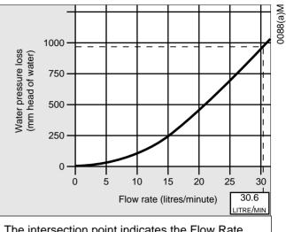
The intersection point indicates the Flow Rate required to achieve 11°C temperature difference.
