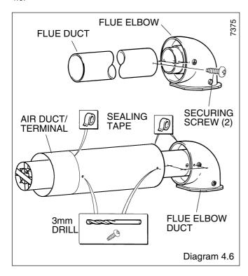
NOTE: The telescopic flue assembly will require drilling.
