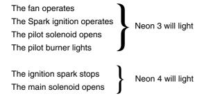
and after a short period of time the main burner will light, look through viewing window, see diagram 8.2.
