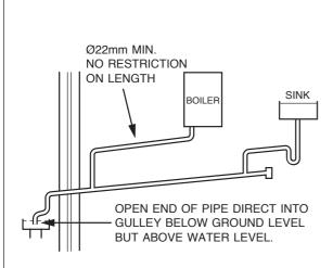
Internal Termination Downstream of Sink Waste
