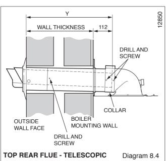
**Top Side flue - Telescopic -** with the flue elbow temporarily fitted, measure the distance from the outside wall to the butt joint, see diagram 8.6. If the measurement 'Y' exceeds 525mm, then the appropriate length of extension pipe is required, if the dimension is less than 320mm DO NOT cut the flue, it can project to a maximum of 600mm, if this is not desirable then a Standard flue MUST be used and cut to length.
