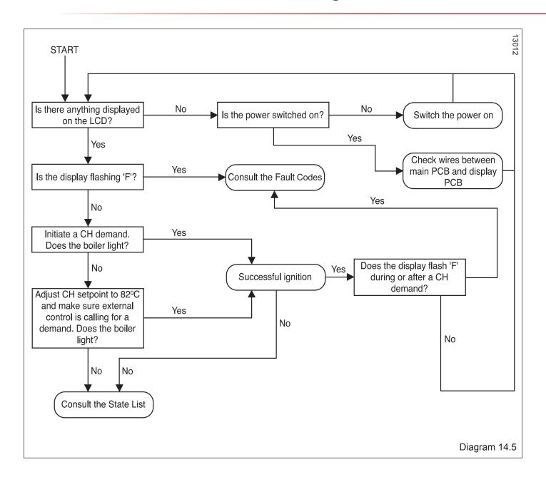
In all circumstances press the reset button to clear the fault. If the fault persists, consult the table below.
