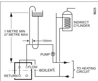
The COLD FEED PIPE may be connected to flow pipe, adjacent to the open vent pipe as shown. (THERE MUST ALWAYS BE A COLD WATER PATH TO THE RETURN CONNECTION OF THE BOILER)
