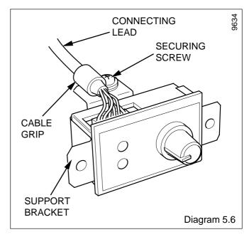
Remove the boiler user control and its long connecting lead from the control box, see diagrams 5.8 and 10.4.
