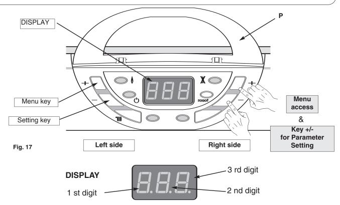
To gain access to setting menus press simultaneously on — and + keys on the Right. side during 5 seconds. (fig. 18). Menu 1 is displayed.
