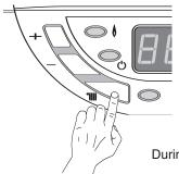
Press on key 29 \* , the green indicator 30 will light and the display will show the Heating flow temperature.
