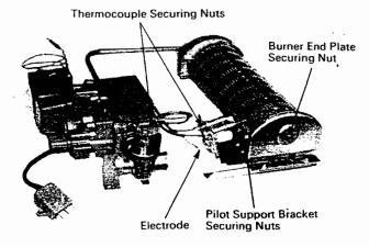
Fig. 18. Burner and Controls (i)
