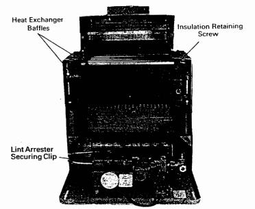
Fig. 17. Combustion Chamber
