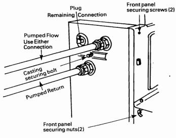
Fig. 6. Fully Pumped System
