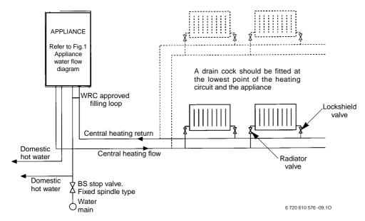
Fig. 5 Sealed primary water system
