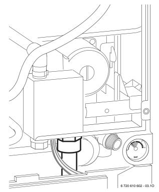
Fig. 11 Position of the condensate drain
