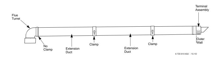
Fig. 18 Flue with extensions
