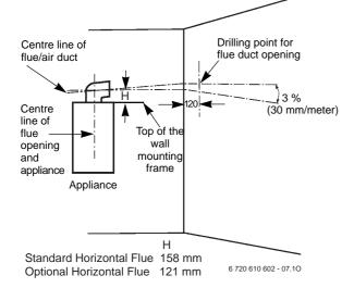
Fig. 15 Marking the position of the side flue opening
