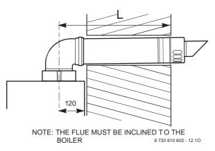
Fig. 20 Flue length - rear
