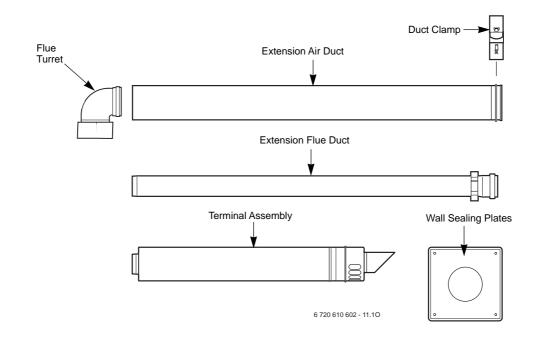
Fig. 19 Flue components
