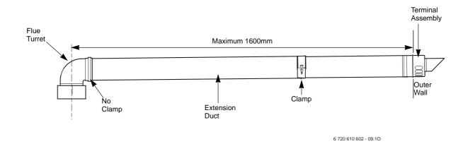
Fig. 17 Flue with one extension
