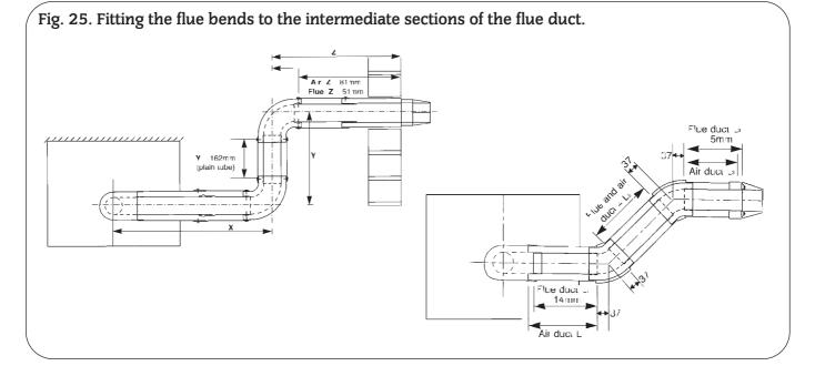
The first, vertical, section (equivalent to dimension X) is measured from the top of the boiler casing. Cut the vertical section of the extension duct to 167mm less than the measured distance. Do not remove the socketed ends.
