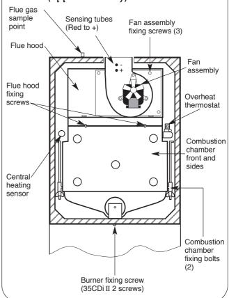
**(f) Flue Hood Assembly.** Remove the fan assembly. Undo the two screws securing the flue hood. Lift and slide the flue hood assembly from the appliance. See Fig. 31. When refitting the hood ensure that the rear return edge passes under the lip at the rear of the combustion chamber.
