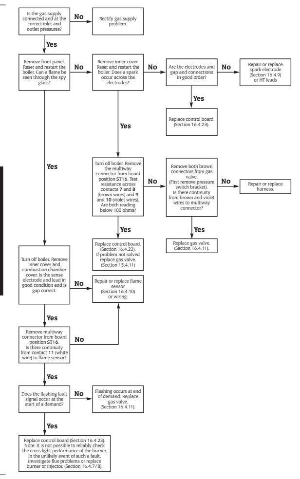
FAIL POINT H "Burner Lockout"
