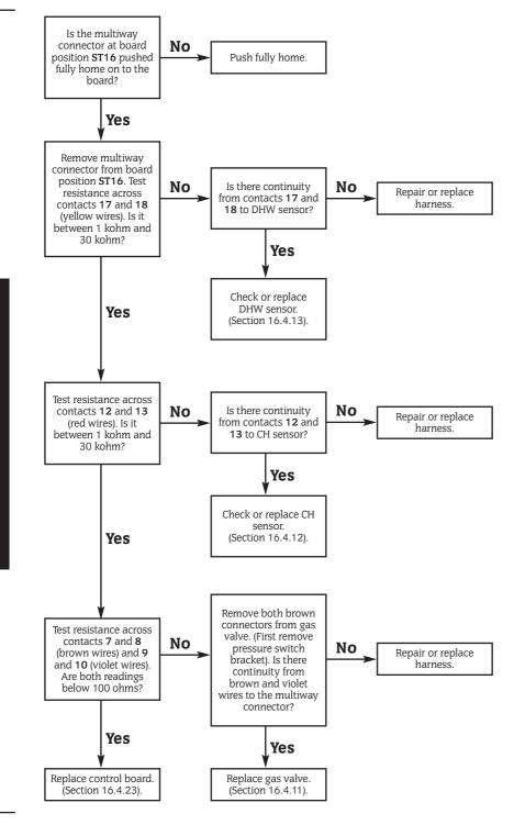
FAIL POINT I "Sensor Fault"
