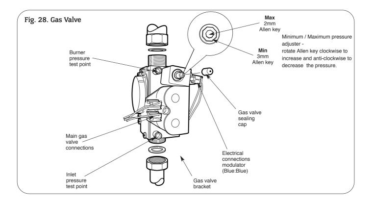
sensed by the control circuit. The burner pressure should be 14.8mbar (24CDi) or 15.5mbar (28CDi) or 13.5mbar (35CDi II) for natural gas and 35.5mbar (24/28CDi) or 34.7mbar (35CDi II) for propane. If the burner pressure cannot be achieved then check that the inlet pressure at the appliance is 20mbar for natural gas and 37mbar for propane. This is equivalent to a 18.5-19.0 mbar (G20) or 36 mbar (G31) at the gas valve. Set the gas valve mode switch to the minimum position.
