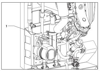
Fig. 8.8 Cleaning the condense trap
