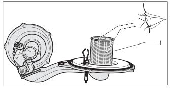
Fig. 8.4 Checking burner
