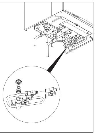
Fig. 5.4 Fitting the pressure relief valve
