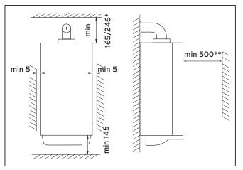
Fig. 4.3 Required minimum gaps/assembly clearances
