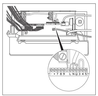
Fig. 5.13 Example for cable routing
