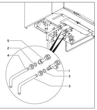
Fig. 5.2 Hot water and cold water connection
