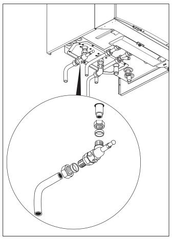
Fig. 5.3 Heating connection
