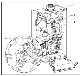
Fig. 8.1 Measuring the CO<sub>2</sub> concentration, specifying the air ratio (gas setting)
