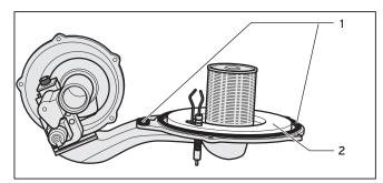
Fig. 8.5 Replacing silicone gaskets
