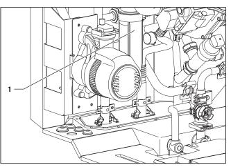
Fig. 6.4 Filling the condense trap
