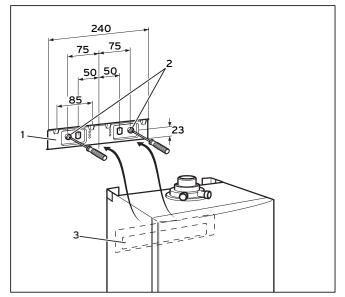
Fig. 4.4 Mounting the appliance
