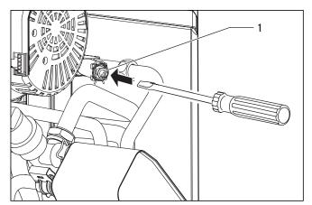
Fig. 7.3. Setting the by-pass valve
