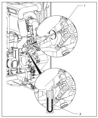
Fig. 6.6 Measuring the gas inlet working pressure
