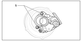
Fig. 10.3 Gas fitting/fan screwed joint
