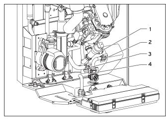
Fig. 8.7 Cleaning the secondary heat exchanger
