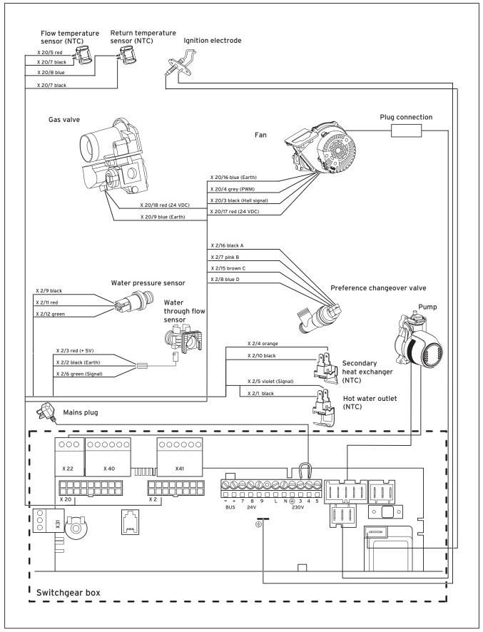
Fig. 5.16 Electronic board layout ecoTEC exclusive
