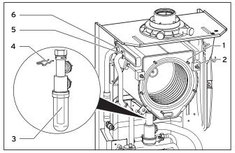
Fig. 10.4 Replacing primary heat exchanger
