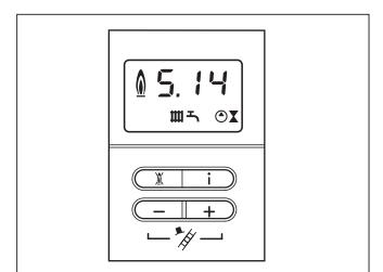
Fig. 6.9 Display during hot water preparation
