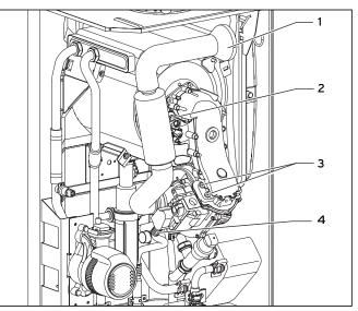
Fig. 10.2 Dismantling fan with gas valve
