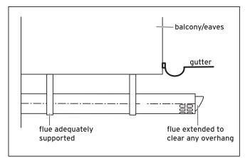
Fig. 5.10 Flue pipe terminating under balconies or gutters
