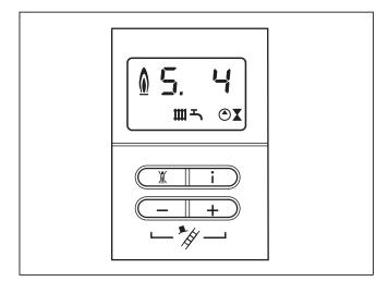
Fig. 6.8 Display during heating mode
