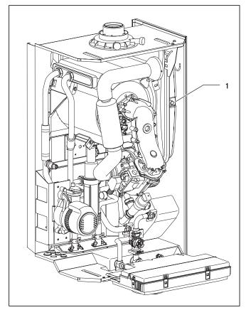
Fig. 8.9 Checking the expansion vessel
