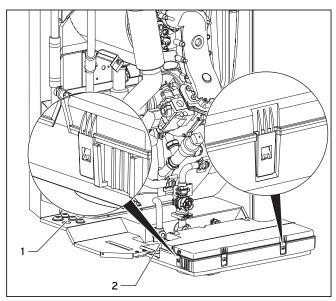
Fig. 5.12 Opening the switchgear box rear wall
