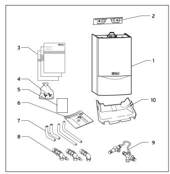
Fig. 4.1 Scope of delivery for ecoTEC exclusive
