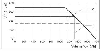
Fig. 7.2 Characteristic pump line for ecoTEC exclusive 832 and 838
