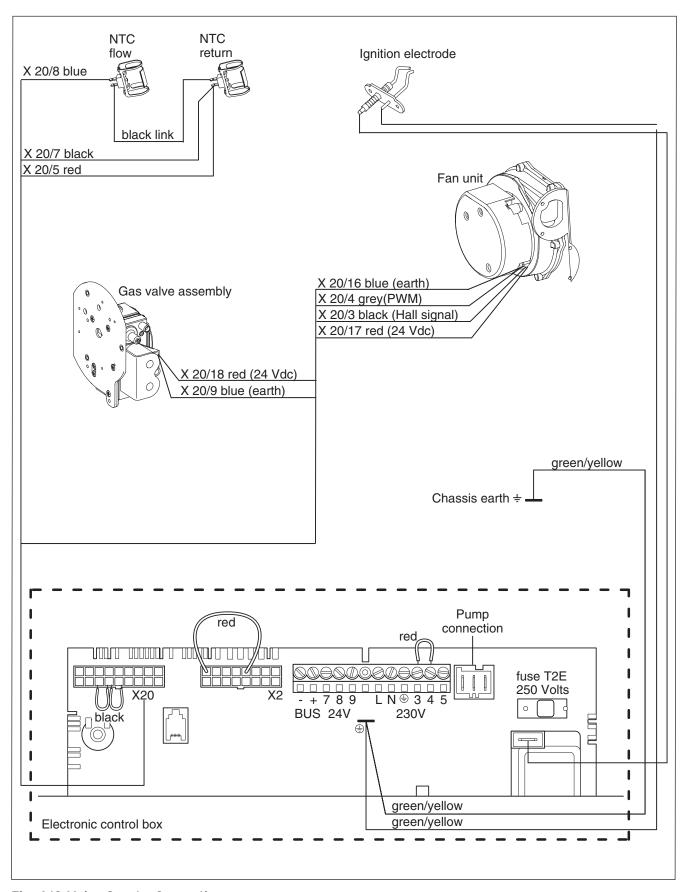
Fig. 4.10 Mains Supply Connection
