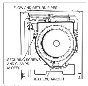
Fig. 11.2 Heat exchanger removal
