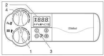
Fig. 5.4 Switching on the appliance
