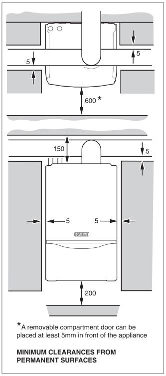
Fig. 4.1 Distance during installation
