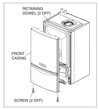
Fig. 4.4 Removing front casing
