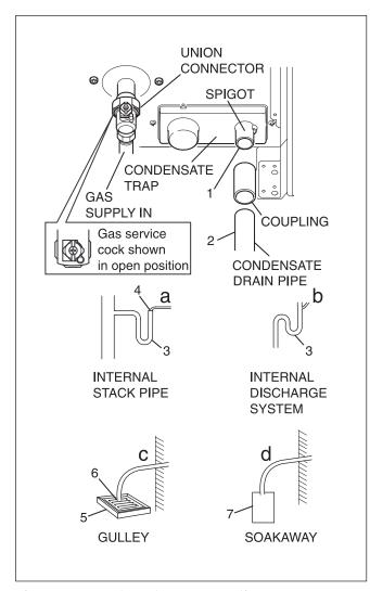
Fig. 4.5 Gas and condense connections
