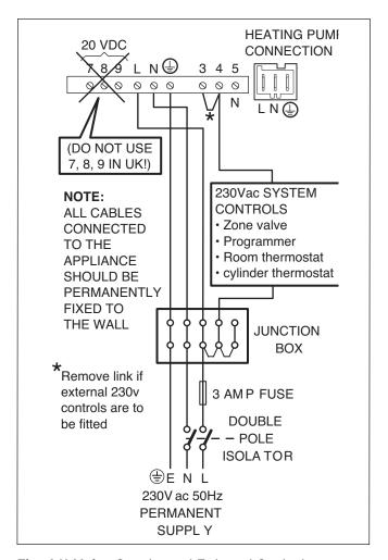
Fig. 4.11 Mains Supply and External Controls
