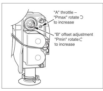
Fig. 9.2 Gas control valve
