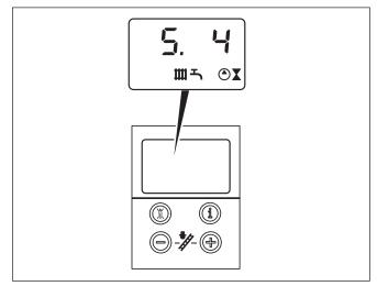
Fig. 7.2 Display indicator during heating mode
