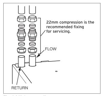
Fig. 4.6 Water connections
