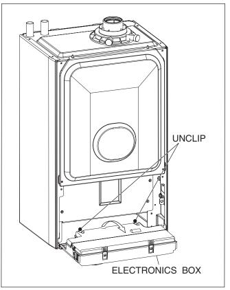
Fig. 4.7 Mains Supply Connection
