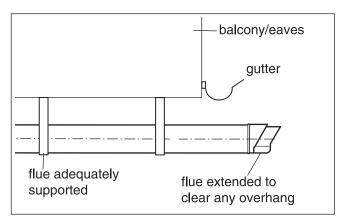
Fig. 3.7 Flue termination under balcony/eves
