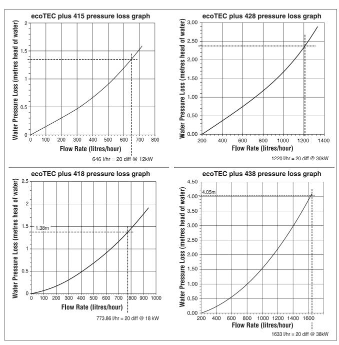
Fig. 3.8 Pressure loss
