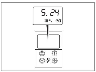
Fig. 7.3 Display indicator during water heating
