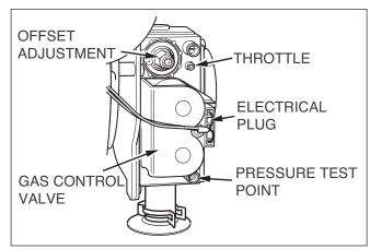
Fig. 5.3 Gas control valve
