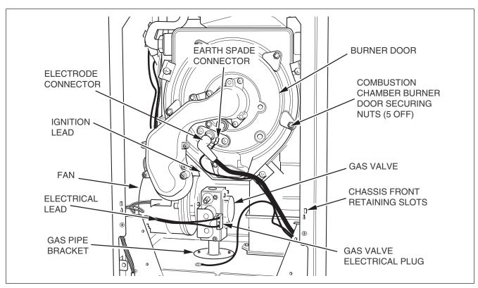
Fig. 8.6 Fan, Gas valve and Burner
