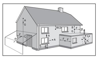
Fig. 3.6 Flue termination
