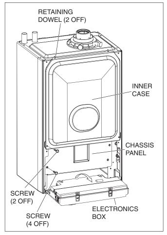
Fig. 5.1 Inner case and chassis removal
