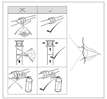
Fig. 7.1 Functional checks (appliance on)
