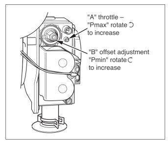
Fig. 6.1 Gas control valve
