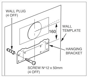
Fig. 4.3 Boiler hanging bracket
