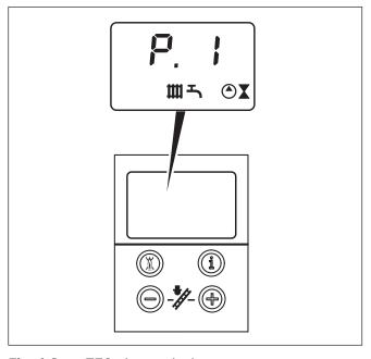
Fig. 6.2 ecoTEC plus controls
