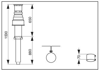
Fig. 3.5 Vertical Flue System Art. No. 303200
