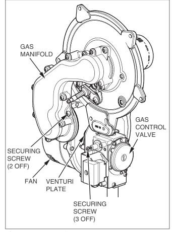
Fig. 11.1 Fan removal
