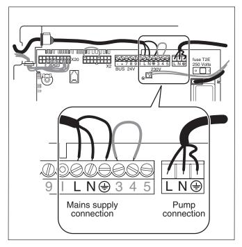
Fig. 4.8 Mains Supply Connection
