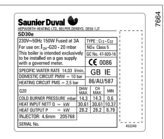
The appliance flue type is a  $\rm C_{12}$  and  $\rm C_{32}$ . This refers to a concentric flue where the fan is downstream of the heat exchanger. The  $\rm C_{12}$  is a horizontal flue termination, and the  $\rm C_{32}$  is a vertical flue termination.
