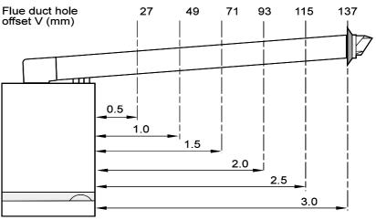
Distance in metres from side of boiler to side wall H (m)
