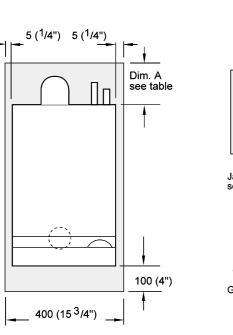
Front clearance: 450mm (17 3/4") from the front of the boiler casing. The minimum front clearance when built in to a cupboard is 5mm (1/4")
