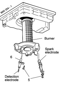
**9.** Check the ignition and operation of the burner.
