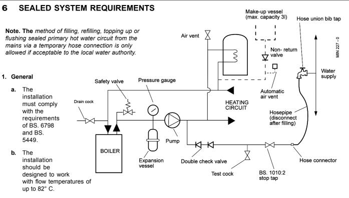
c. All components of the system, including the heat exchanger of the indirect cylinder, must be suitable for a working pressure of 3 bar (45lb/in<sup>2</sup>) and temperature of 110°C. Care should be taken in making all connections so that the risk of leakage is minimised.
