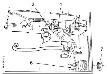
**Note.** Take care not to damage the thermostat capillary when inserting it into the pocket.
