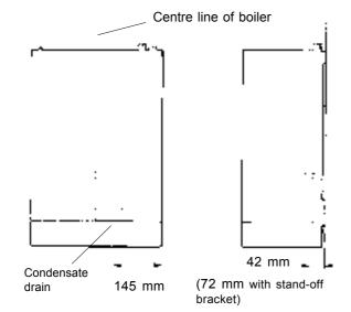
**Note.** The drain connection is located at the rear of the controls compartment.
