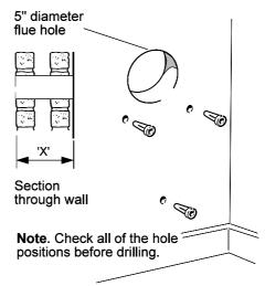
Note. If the terminal is to be sited within 25-40mm of a corner or vertical pipe (refer to Table 3) then the hole MUST be accurately cut and the rubber weather seal trimmed around the groove provided. The terminal wall plate need not be fitted.
