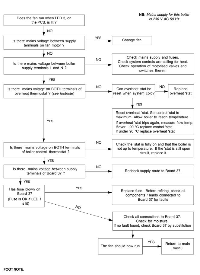
Presence of live supply on a terminal may be checked with a multimeter set to the appropriate AC range (apply the other probe of the meter to Mains neutral, e.g. on terminal N of the incoming supply).
