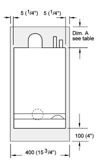
Front clearance: 450mm (17 3/4") from the front of the boiler casing. The minimum front clearance when built in to a cupboard is 5mm (1/4")
