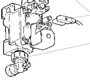
**8.** Undo the two extended nuts retaining the gas injection pipe and withdraw the pipe, taking care not to lose the O ring seal.
