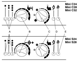
12 Press and hold the reset button D for about 10 seconds until the lock-out signal lamp E blinks.
