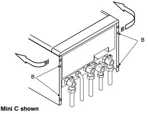
5 Remove the screws C and remove the boiler inner casing.
