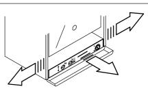
When completely pulled out, the panel can rotate 45° downwards to facilitate the operations on the internal parts.
