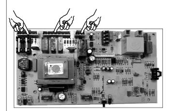
6 To disconnect the connectors indicated in the next figure, delicately press the hook present on one side of each socket.
