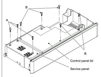
5 Remove all the wiring connected to the main control p.c.b. To disconnect the connectors indicated, delicately flex the hook present on one side of each socket.
