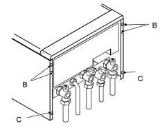
4 Remove the side panels or move the lower part of the side panels and pull the control panel.
