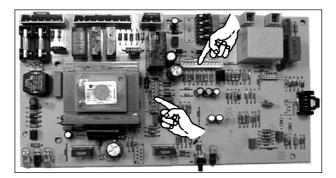
7 Remove the spindles of the two control knobs by delicately pulling them with pliers in the direction shown by the arrows.
