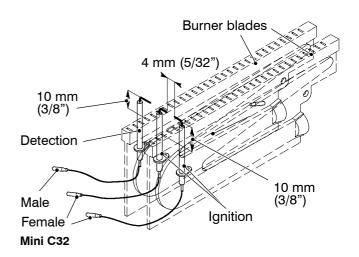
9 Check that the spark and detection electrodes leads are in good condition and renew as necessary.
