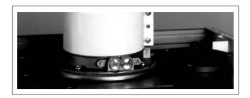
Using the especially designed apertures, readings can be taken on the temperature of the combustion by-products and of the combustion air, as well as of the concentrations of  $O_2$  and  $CO_2$ , etc.
