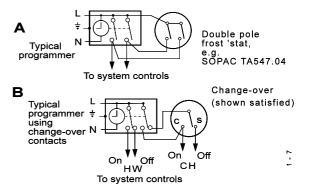
**Diagram A** shows a double pole frost thermostat, which should suffice for all systems which do not use the OFF terminals of the programmer.
