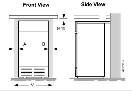
Note. 3/100P ONLY. If minimum LH side clearance is used, the TTB downdraught thermostat and bracket should be moved to the RH side of the boiler (alternative location).
