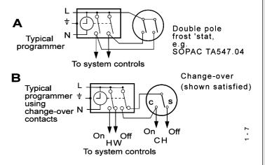
**Diagram A** shows a double pole frost thermostat, which should suffice for all systems which do not use the OFF terminals of the programmer.
