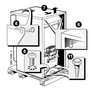
**11.** The boiler is held to the packaging base by 4 M6 hex head screws. Remove the front screws, slacken the rear screws and remove the boiler from the packaging base.
