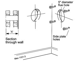
Note. If the terminal is to be sited within 25-40mm of a corner or vertical pipe (refer to Table 3) then the hole MUST be accurately cut and the rubber weather seal trimmed around the groove provided. The terminal wall plate need not be fitted.
