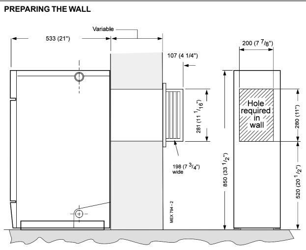
1. Cut the appropriate hole in the wall for insertion of the terminal assembly.
