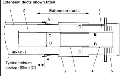
1. BEFORE PLACING THE BOILER IN POSITION, loosely fit the extension air duct and terminal assembly to the boiler air duct and adjust to the required overall duct length.
