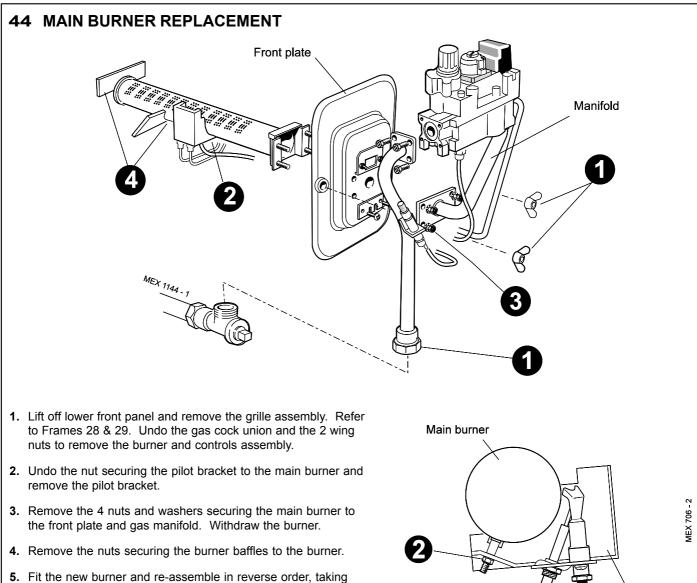
care not to damage the main burner injector, which is screwed into the end of the gas manifold.
