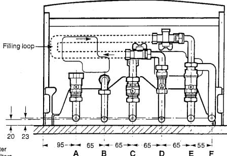
Note: Disconnect the filling loop after filling the central heating system.
