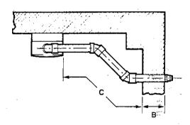
$L = B + C + 180 \text{ mm} + (2 \times 45^{\circ} \text{ bends} = 1 \text{ metre})$
