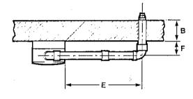
$L = B + E + F + 180 \text{ mm} + (90^{\circ} \text{ bend} = 1 \text{ metre})$
